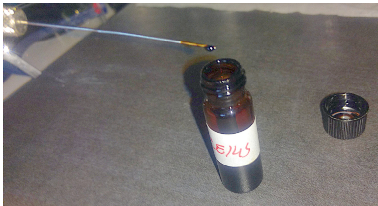
Figure 6.2.1: Photograph of the pure medium-heavy crude oil residue sample sent by the WG Schrader. The sample is brownish-black, viscous, and has a slight smell.
