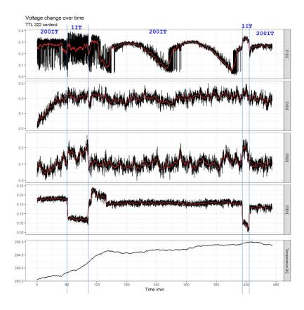
Comparison with Keithley precision multimeter Labjack is a lot less precise. This shows that Keithley should be used for absolute values while the divider is more suitable for shifts in time.
